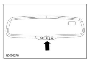
3. Momentarily press and release the MODE button to increase the zone increment by one. Set the zone display number to match the vehicle location that is shown on the compass calibration zone map.
